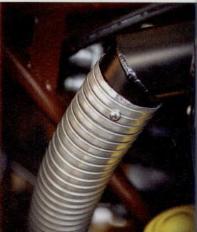
METICULOUS FABRIC WORK is a Roger Meggers specialty, and no the original Super Cub restoration, the Meggers went totally original and even made metal air ducting (bottom right) instead of using readily available modern materials.
